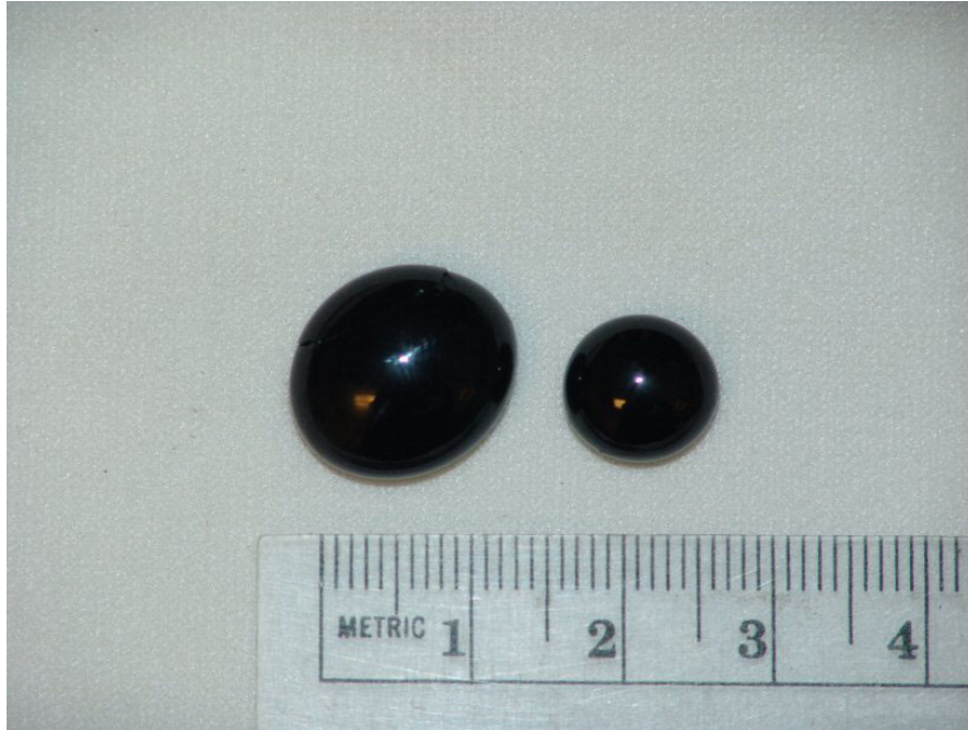
Figure 10. Bulk glass samples cast from JSC-1 lunar regolith simulant
