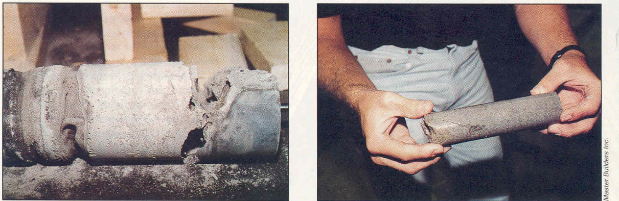
Figure 8. Concrete Samples Prepared in Microgravity Environments [Bury, et al. 1995]
